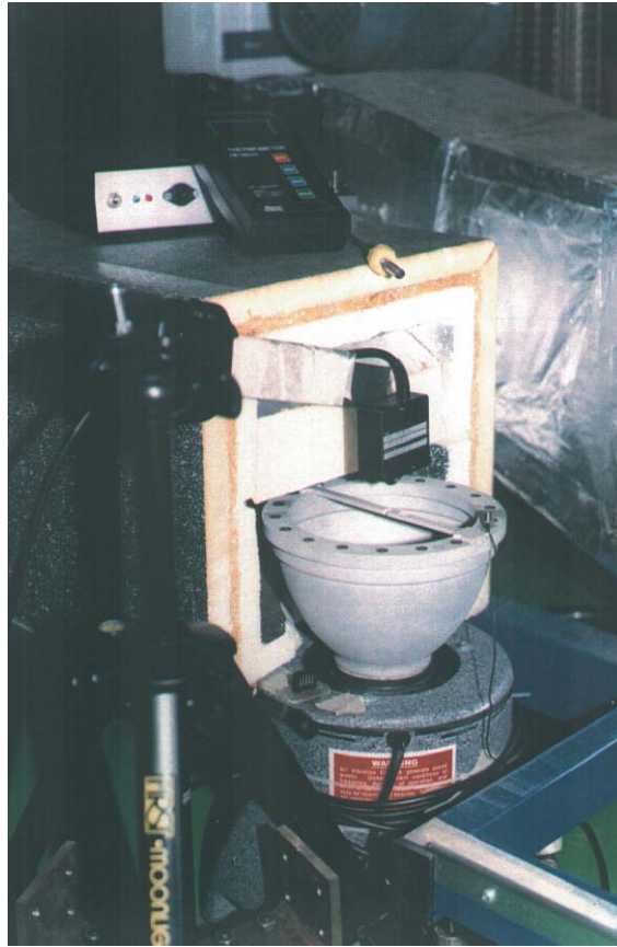
Fig. 8. Photograph of the experimental set-up for measurement of Young's modulus.
